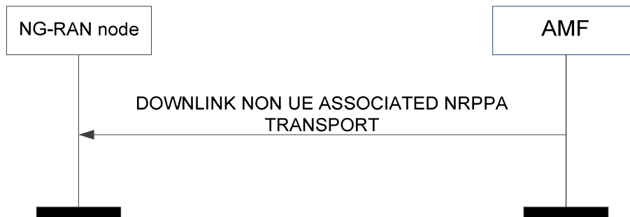
Figure 8.10.2.3-1: Downlink non UE-associated NRPPa transport
