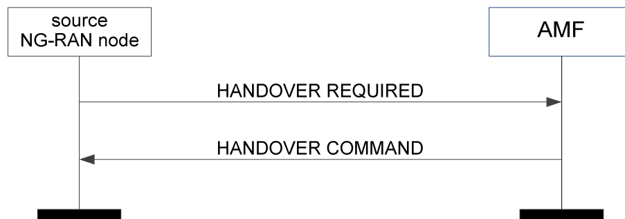
Figure 8.4.1.2-1: Handover preparation: successful operation
