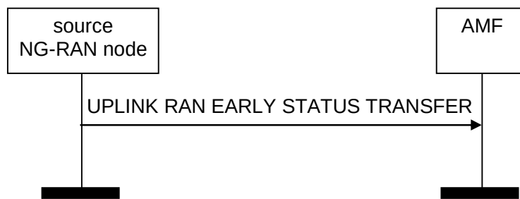
Figure 8.4.9.2-1: Uplink RAN Early Status Transfer
