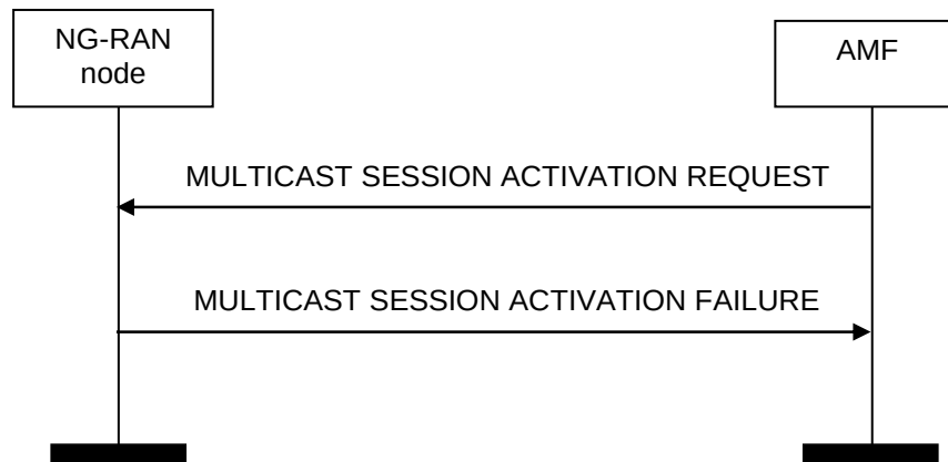
Figure 8.18.3.3-1: Multicast Session Activation, unsuccessful operation.
