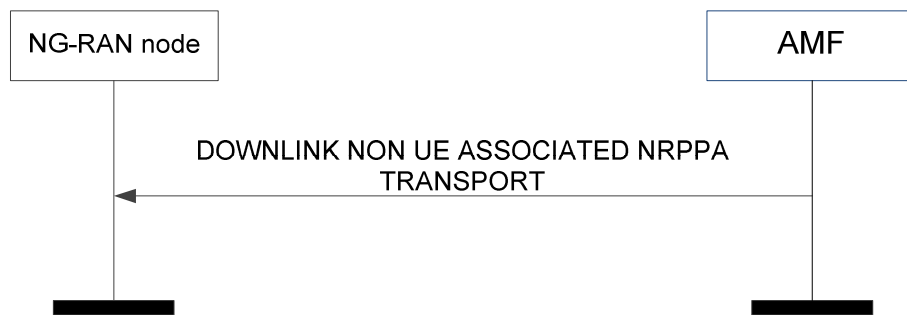
Figure 8.10.2.3-1: Downlink non UE-associated NRPPa transport
