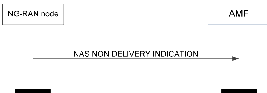
Figure 8.6.4.2-1: NAS non delivery indication
