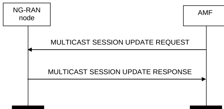
Figure 8.18.5.2-1: Multicast Session Update, successful operation.
