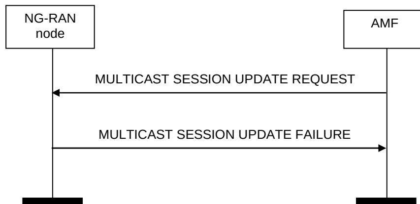
Figure 8.18.5.3-1: Multicast Session Update, unsuccessful operation.
