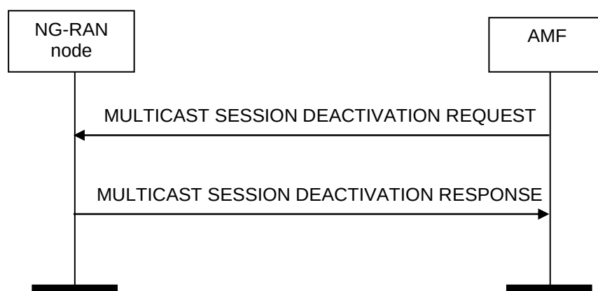
Figure 8.18.4.2-1: Multicast Session Deactivation, successful operation.
