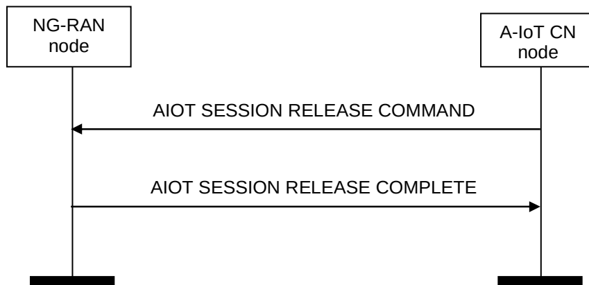
Figure 8.20.4.2-1: A-IoT Session Release, successful operation.
