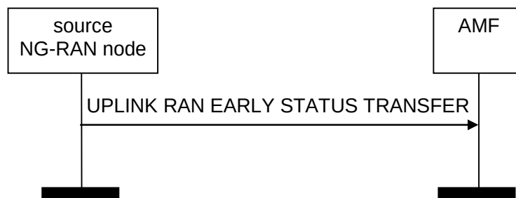
Figure 8.4.9.2-1: Uplink RAN Early Status Transfer
