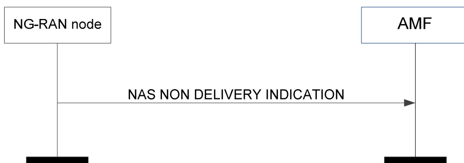
Figure 8.6.4.2-1: NAS non delivery indication
