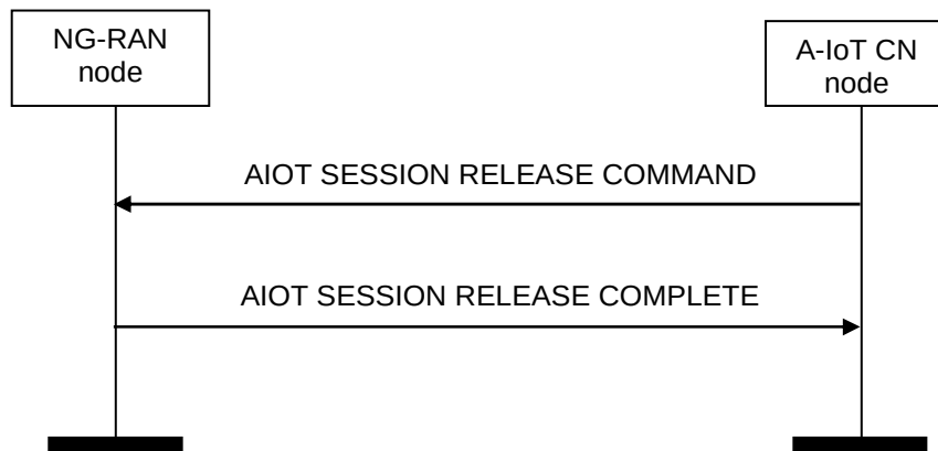
Figure 8.20.4.2-1: A-IoT Session Release, successful operation.
