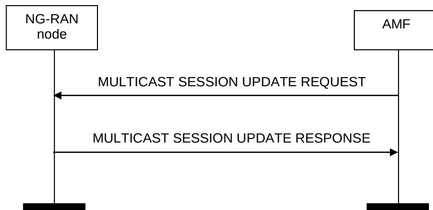
Figure 8.18.5.2-1: Multicast Session Update, successful operation.
