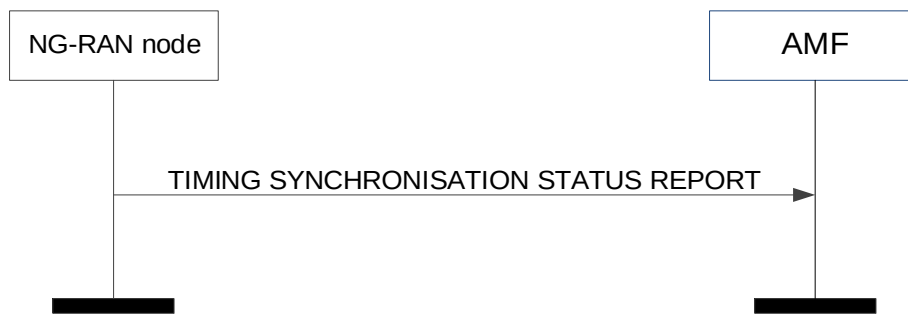
Figure 8.19.2.2-1: Timing synchronisation status report
