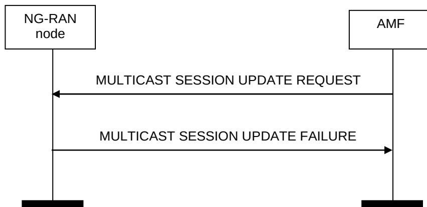
Figure 8.18.5.3-1: Multicast Session Update, unsuccessful operation.
