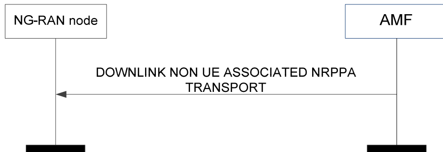
Figure 8.10.2.3-1: Downlink non UE-associated NRPPa transport
