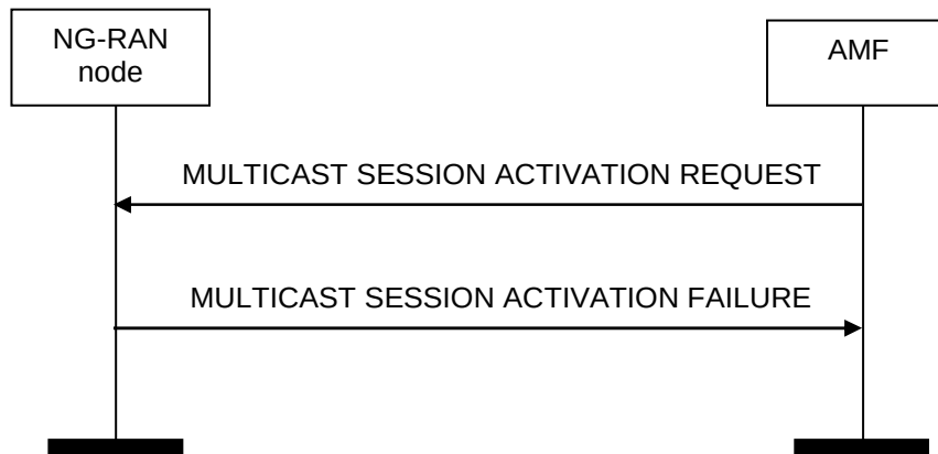
Figure 8.18.3.3-1: Multicast Session Activation, unsuccessful operation.
