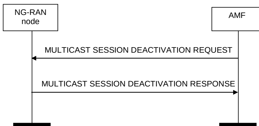
Figure 8.18.4.2-1: Multicast Session Deactivation, successful operation.
