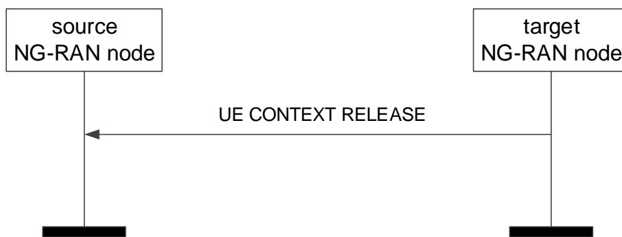
Figure 8.2.7.2-1: UE Context Release, successful operation for handover
