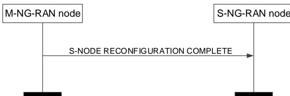
Figure 8.3.2.2-1: S-NG-RAN node Reconfiguration Complete procedure, successful operation.
