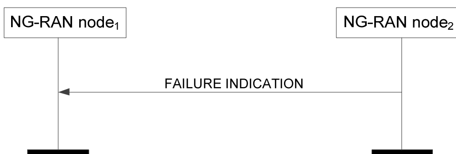
Figure 8.4.7.2-1: Failure Indication, successful operation
