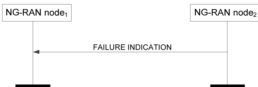
Figure 8.4.7.2-1: Failure Indication, successful operation
