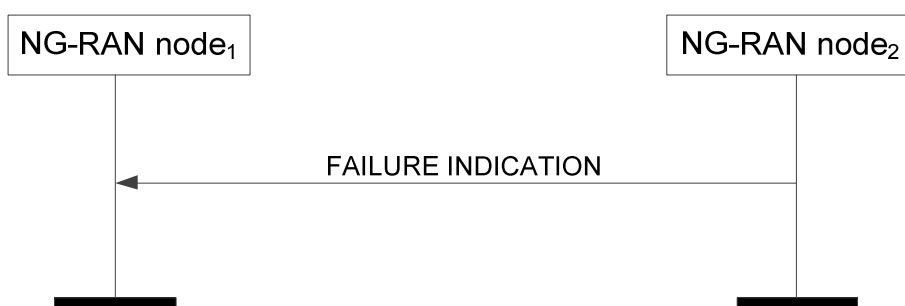
Figure 8.4.7.2-1: Failure Indication, successful operation
