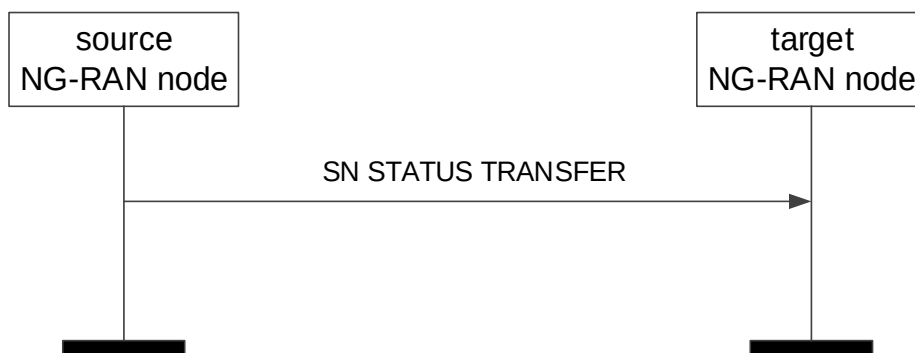
Figure 8.2.2.2-1: SN Status Transfer, successful operation
