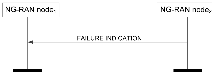
Figure 8.4.7.2-1: Failure Indication, successful operation
