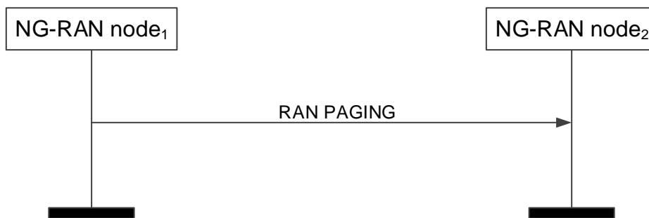
Figure 8.2.5.2-1: RAN Paging: successful operation
