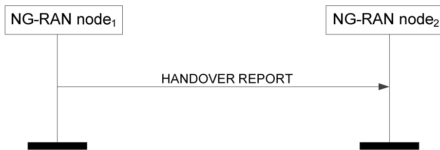
Figure 8.4.8.2-1: Handover Report, successful operation
