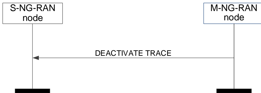
Figure 8.3.15.2-1: Deactivate Trace, successful operation
