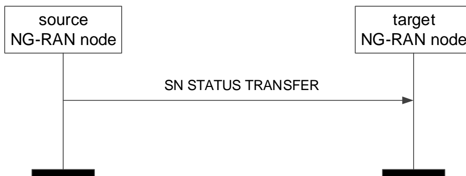
Figure 8.2.2.2-1: SN Status Transfer, successful operation
