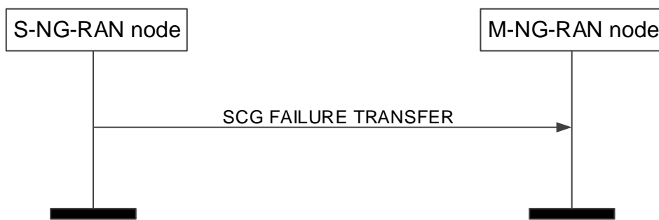
Figure 8.3.18.2-1: SCG Failure Information Transfer, successful operation
