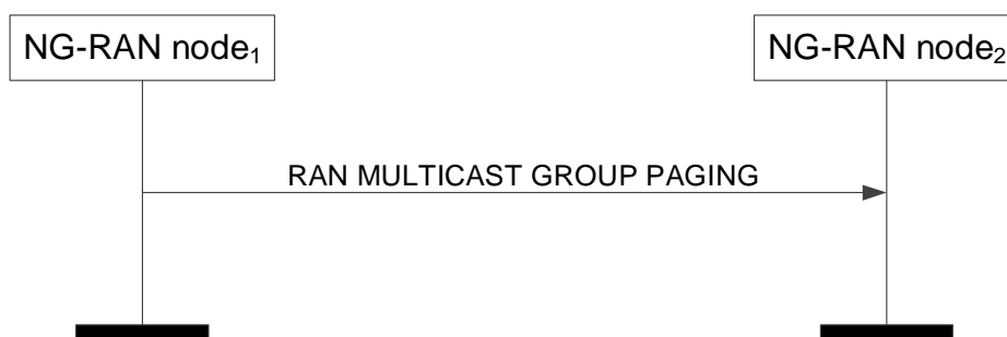
Figure 8.2.11.2-1: RAN Multicast Group Paging, successful operation
