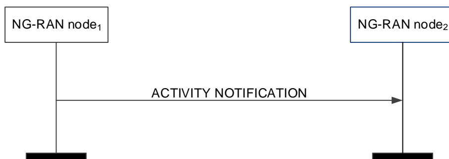
Figure 8.3.11.2-1: Activity Notification, successful operation
