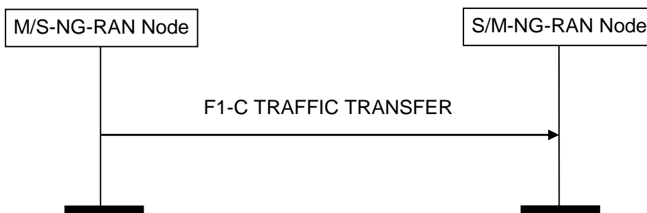
Figure 8.5.1.2-1: F1-C Traffic Transfer procedure, successful operation
