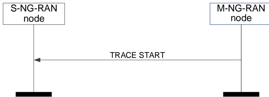
Figure 8.3.14.2-1: Trace Start, successful operation
