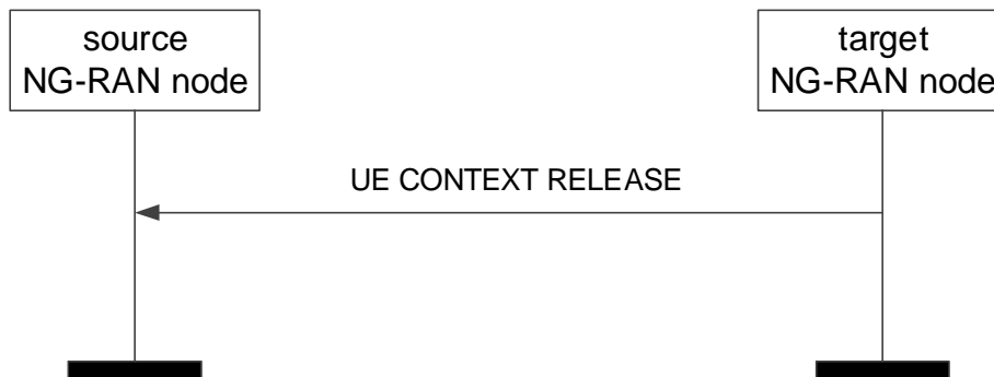
Figure 8.2.7.2-1: UE Context Release, successful operation for handover
