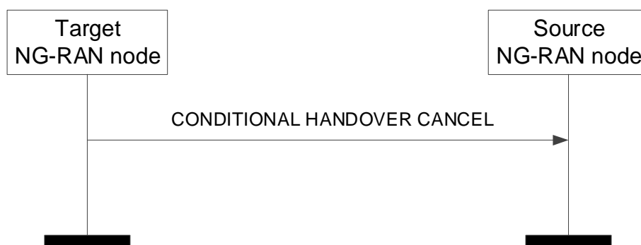
Figure 8.2.9.2-1: Conditional Handover Cancel, successful operation
