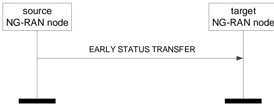
Figure 8.2.10.2-1: Early Status Transfer during DAPS Handover or Conditional Handover, successful operation
