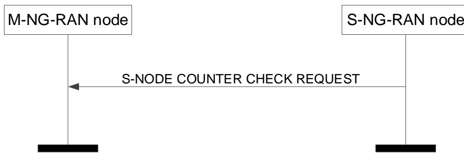
Figure 8.3.8.2-1: S-NG-RAN node Counter Check procedure, successful operation.
