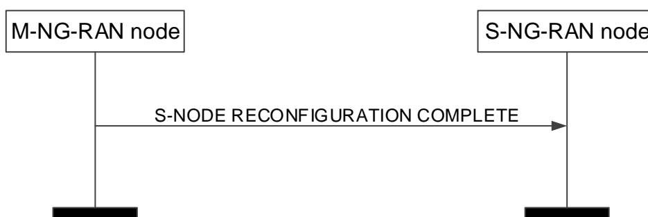
Figure 8.3.2.2-1: S-NG-RAN node Reconfiguration Complete procedure, successful operation.
