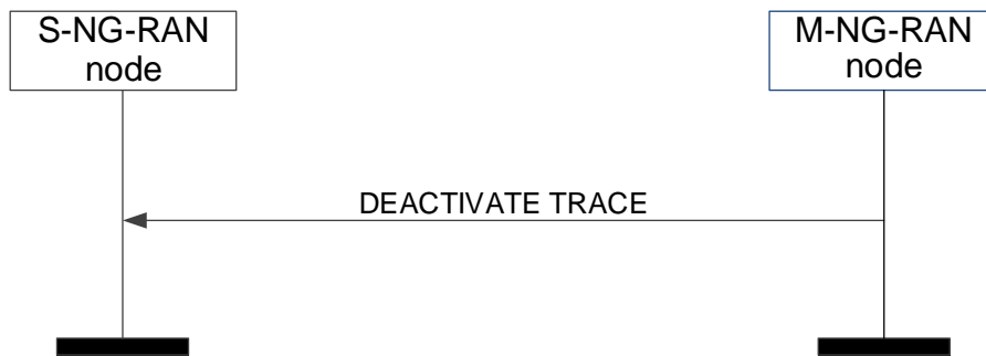
Figure 8.3.15.2-1: Deactivate Trace, successful operation
