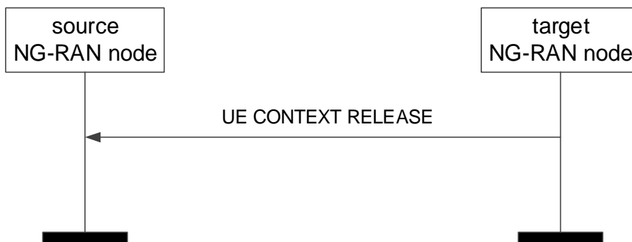
Figure 8.2.7.2-1: UE Context Release, successful operation for handover
