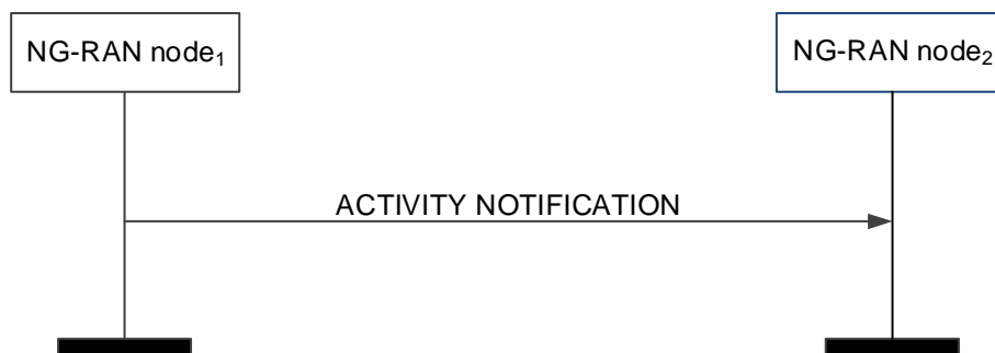
Figure 8.3.11.2-1: Activity Notification, successful operation
