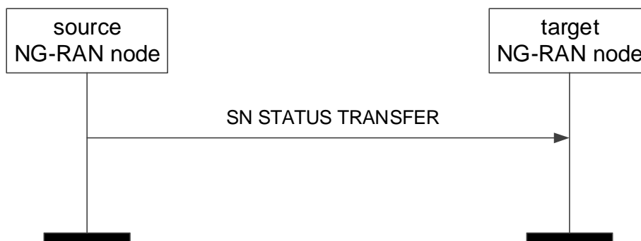
Figure 8.2.2.2-1: SN Status Transfer, successful operation
