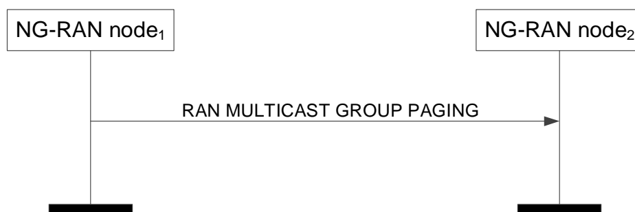
Figure 8.2.11.2-1: RAN Multicast Group Paging, successful operation
