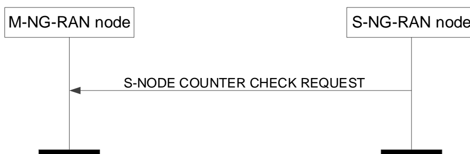
Figure 8.3.8.2-1: S-NG-RAN node Counter Check procedure, successful operation.
