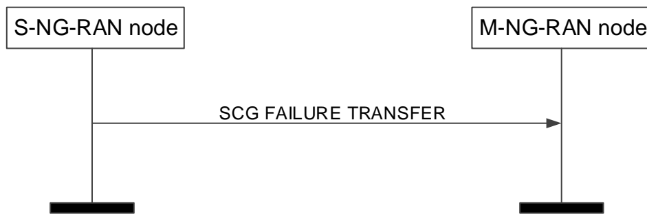
Figure 8.3.18.2-1: SCG Failure Information Transfer, successful operation
