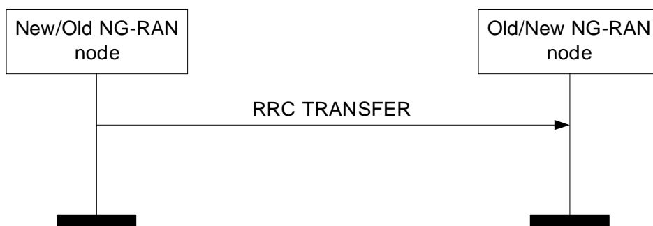
Figure 8.3.9.2-2: RRC Transfer procedure for SDT, successful operation.
