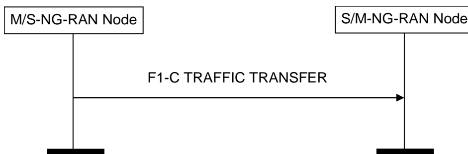
Figure 8.5.1.2-1: F1-C Traffic Transfer procedure, successful operation
