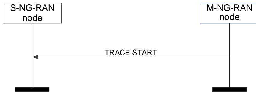
Figure 8.3.14.2-1: Trace Start, successful operation
