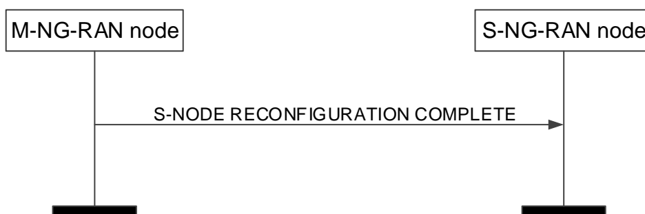
Figure 8.3.2.2-1: S-NG-RAN node Reconfiguration Complete procedure, successful operation.
