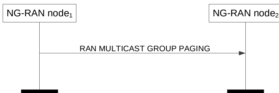
Figure 8.2.11.2-1: RAN Multicast Group Paging, successful operation
