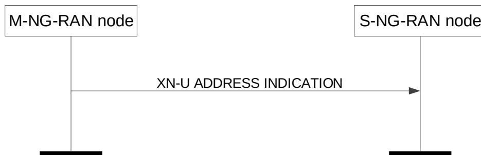
Figure 8.2.6.2-2: Xn-U Address Indication, successful operation for MR-DC with 5GC
