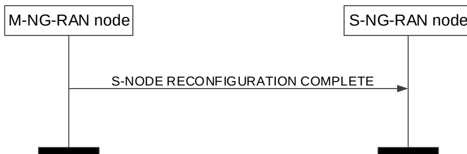
Figure 8.3.2.2-1: S-NG-RAN node Reconfiguration Complete procedure, successful operation.
