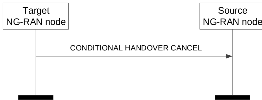
Figure 8.2.9.2-1: Conditional Handover Cancel, successful operation
