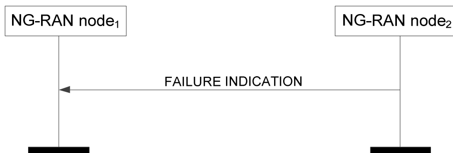
Figure 8.4.7.2-1: Failure Indication, successful operation
