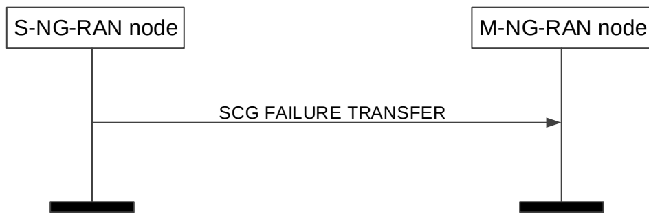
Figure 8.3.18.2-1: SCG Failure Information Transfer, successful operation
