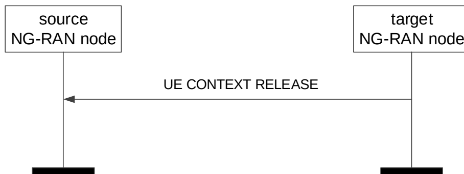
Figure 8.2.7.2-1: UE Context Release, successful operation for handover
