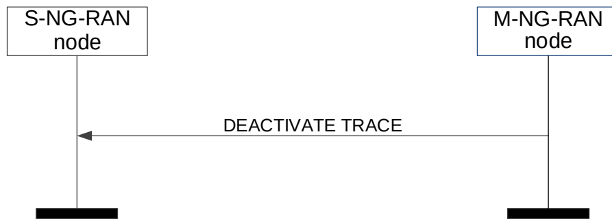
Figure 8.3.15.2-1: Deactivate Trace, successful operation
