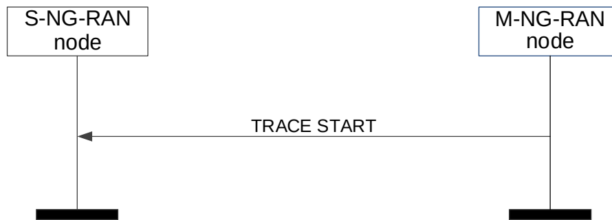
Figure 8.3.14.2-1: Trace Start, successful operation
