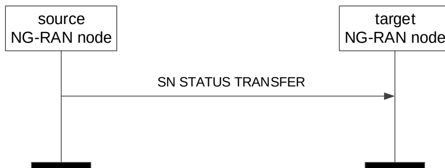
Figure 8.2.2.2-1: SN Status Transfer, successful operation
