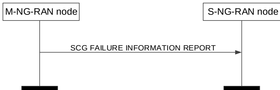
Figure 8.3.17.2-1: SCG Failure Information Report, successful operation
