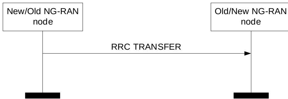
Figure 8.3.9.2-2: RRC Transfer procedure for SDT, successful operation.
