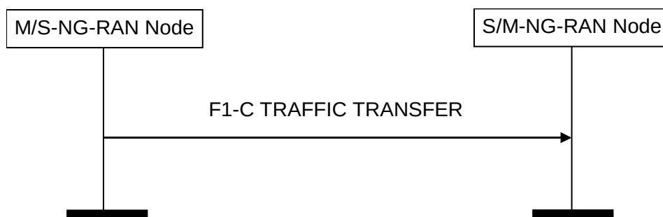
Figure 8.5.1.2-1: F1-C Traffic Transfer procedure, successful operation
