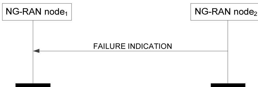
Figure 8.4.7.2-1: Failure Indication, successful operation
