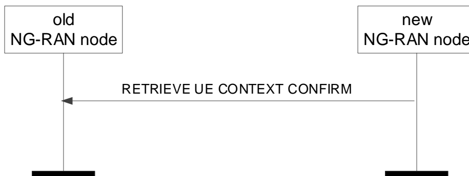
Figure 8.2.12.2-1: Retrieve UE Context Confirm, successful operation
