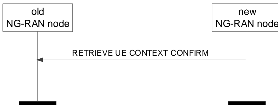
Figure 8.2.12.2-1: Retrieve UE Context Confirm, successful operation
