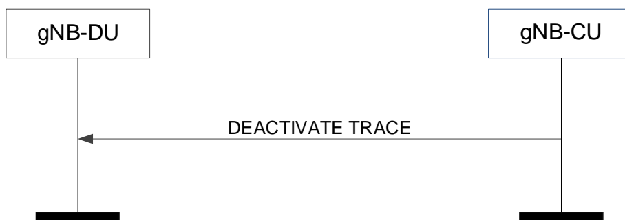
Figure 8.8.2.2-1: Deactivate trace procedure: Successful Operation
