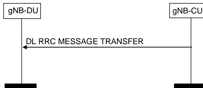
Figure 8.4.2.2-1: DL RRC Message Transfer procedure
