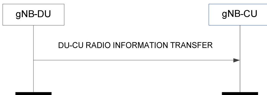
Figure 8.9.1.2-1: DU-CU Radio Information Transfer procedure.
