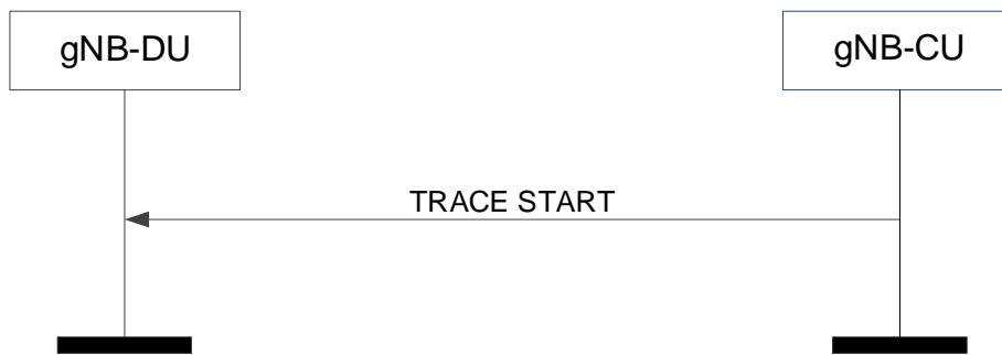
Figure 8.8.1.2-1: Trace start procedure: Successful Operation.
