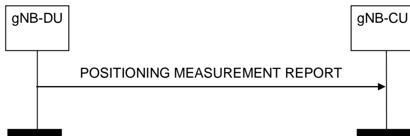
Figure 8.13.4.2-1: Positioning Measurement Report procedure: successful operation
