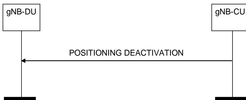
Figure 8.13.11.2-1: Positioning Deactivation procedure, successful operation
