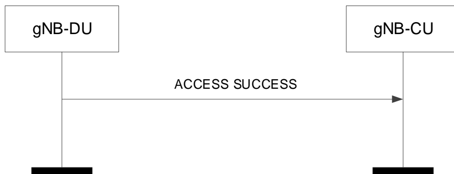
Figure 8.3.8.2-1: Access Success procedure. Successful operation.
