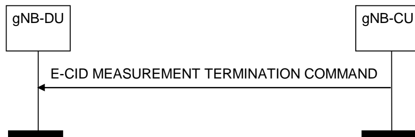
Figure 8.13.15.2-1: E-CID Measurement Termination procedure, successful operation
