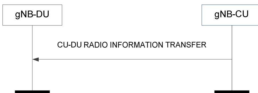
Figure 8.9.2.2-1: CU-DU Radio Information Transfer procedure.
