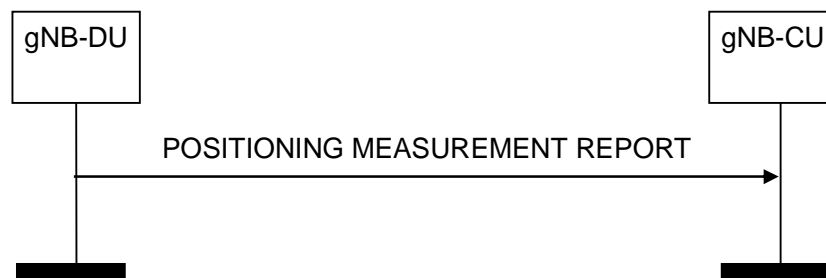
Figure 8.13.4.2-1: Positioning Measurement Report procedure: successful operation
