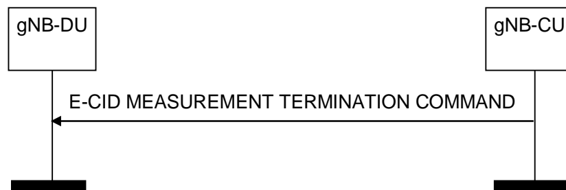
Figure 8.13.15.2-1: E-CID Measurement Termination procedure, successful operation
