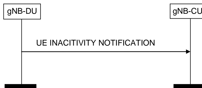
Figure 8.3.6.2-1: UE Inactivity Notification procedure.
