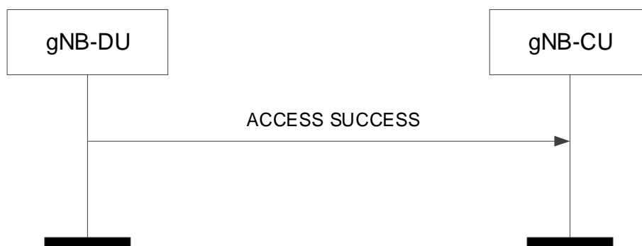
Figure 8.3.8.2-1: Access Success procedure. Successful operation.
