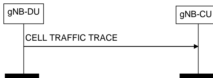
Figure 8.8.3.2-1: Cell Traffic Trace procedure. Successful operation.
