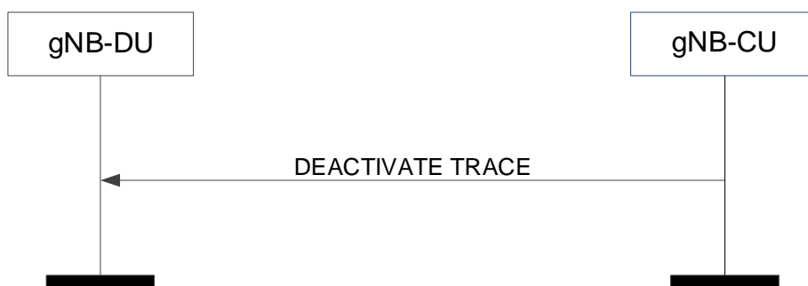
Figure 8.8.2.2-1: Deactivate trace procedure: Successful Operation
