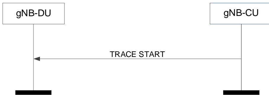
Figure 8.8.1.2-1: Trace start procedure: Successful Operation.
