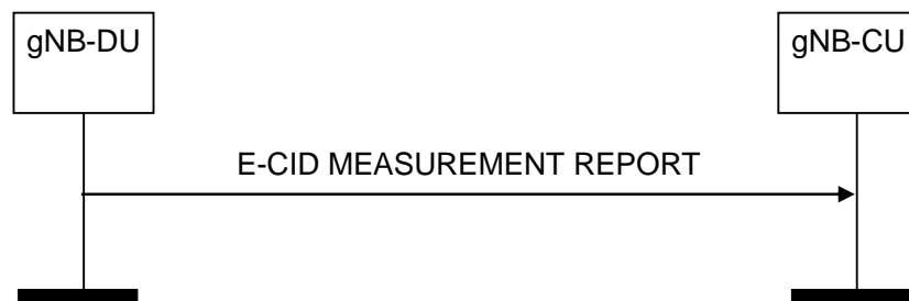
Figure 8.13.14.2-1: E-CID Measurement Report procedure, successful operation
