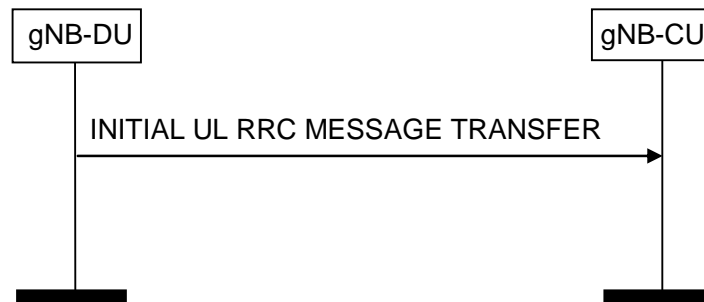
Figure 8.4.1.2-1: Initial UL RRC Message Transfer procedure.
