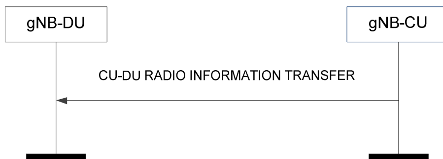
Figure 8.9.2.2-1: CU-DU Radio Information Transfer procedure.
