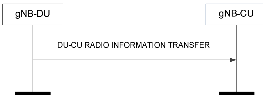
Figure 8.9.1.2-1: DU-CU Radio Information Transfer procedure.
