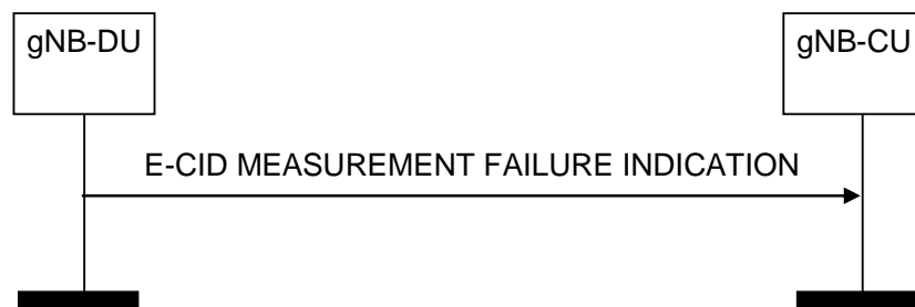
Figure 8.13.13.2-1: E-CID Measurement Failure Indication, successful operation
