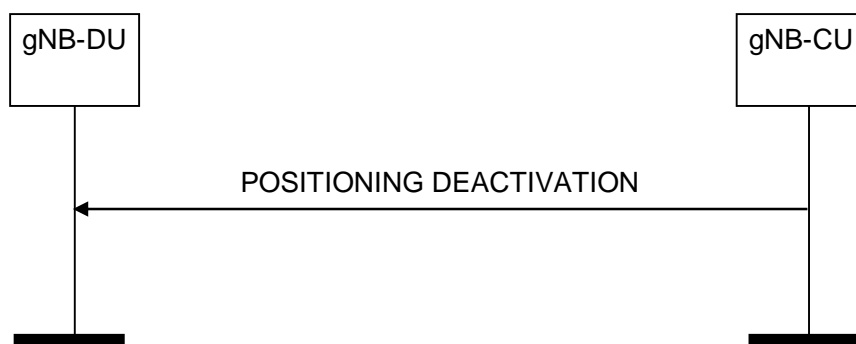
Figure 8.13.11.2-1: Positioning Deactivation procedure, successful operation
