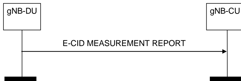
Figure 8.13.14.2-1: E-CID Measurement Report procedure, successful operation
