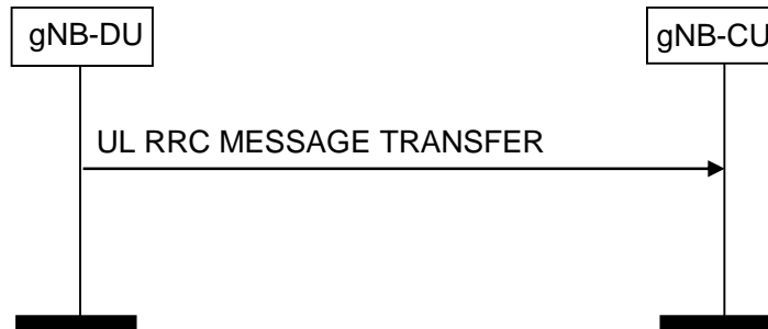
Figure 8.4.3.2-1: UL RRC Message Transfer procedure
