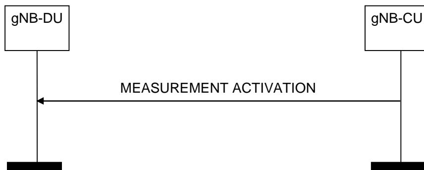
Figure 8.13.19.2-1: Measurement Activation procedure, successful operation
