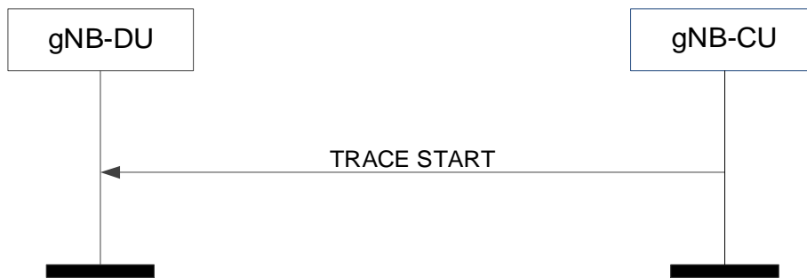
Figure 8.8.1.2-1: Trace start procedure: Successful Operation.
