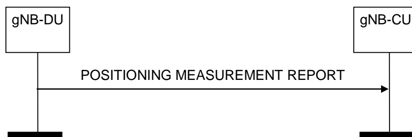
Figure 8.13.4.2-1: Positioning Measurement Report procedure: successful operation
