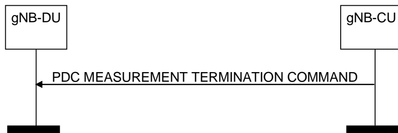
Figure 8.15.3.2-1: PDC Measurement Termination procedure: successful operation
