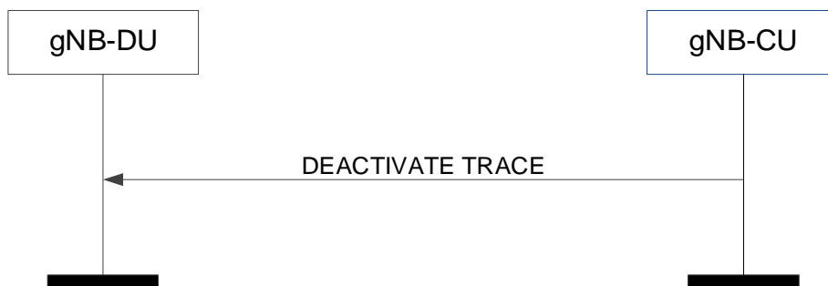
Figure 8.8.2.2-1: Deactivate trace procedure: Successful Operation
