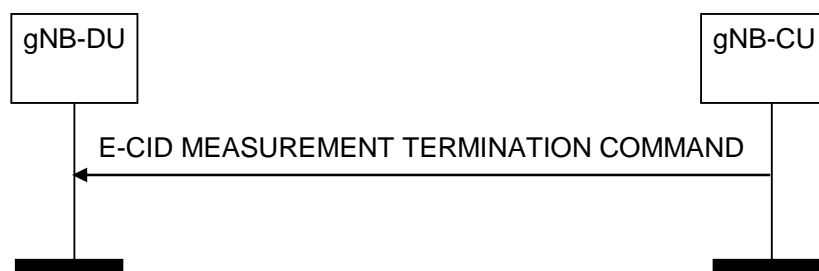
Figure 8.13.15.2-1: E-CID Measurement Termination procedure, successful operation
