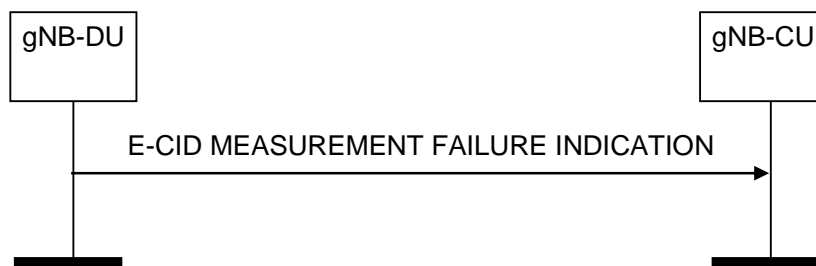
Figure 8.13.13.2-1: E-CID Measurement Failure Indication, successful operation
