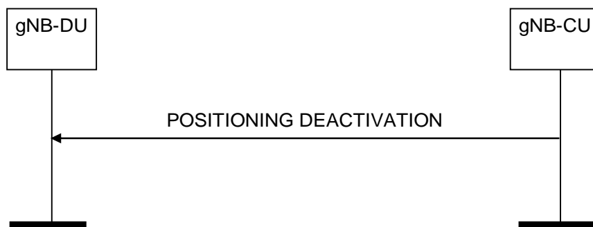
Figure 8.13.11.2-1: Positioning Deactivation procedure, successful operation
