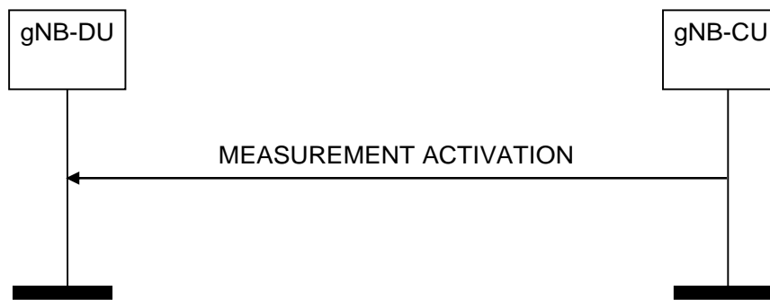
Figure 8.13.19.2-1: Measurement Activation procedure, successful operation
