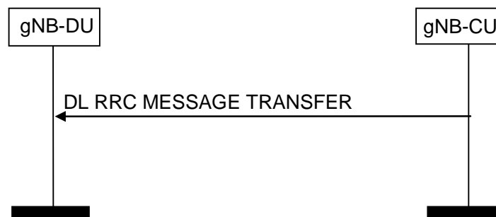
Figure 8.4.2.2-1: DL RRC Message Transfer procedure
