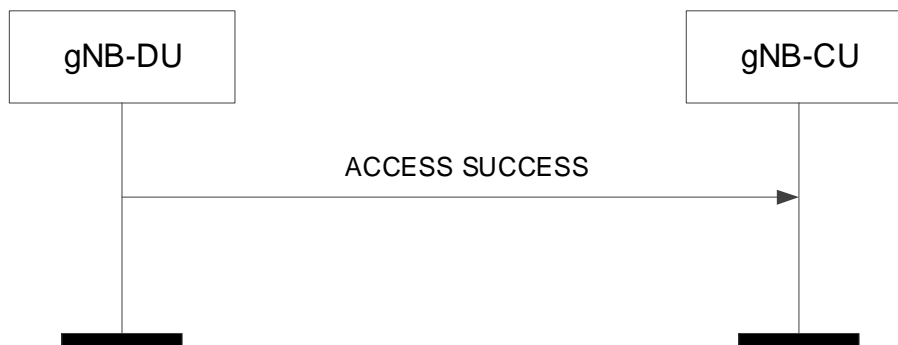
Figure 8.3.8.2-1: Access Success procedure. Successful operation.
