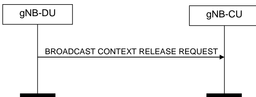
Figure 8.14.3.2-1: Broadcast Context Release Request procedure. Successful operation
