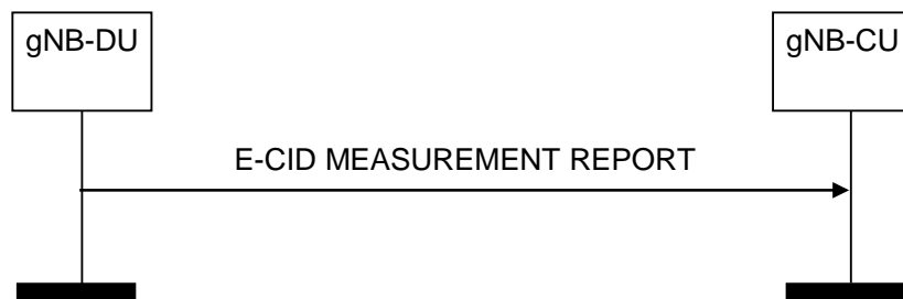
Figure 8.13.14.2-1: E-CID Measurement Report procedure, successful operation
