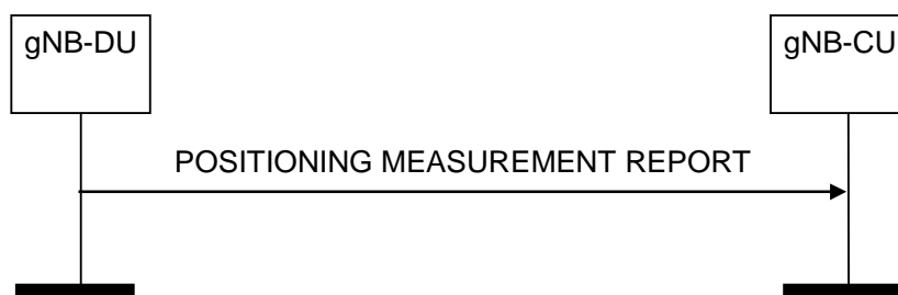
Figure 8.13.4.2-1: Positioning Measurement Report procedure: successful operation
