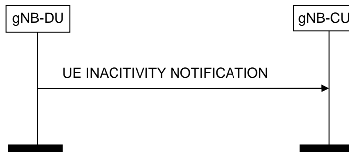
Figure 8.3.6.2-1: UE Inactivity Notification procedure.
