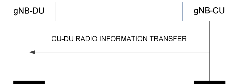
Figure 8.9.2.2-1: CU-DU Radio Information Transfer procedure.
