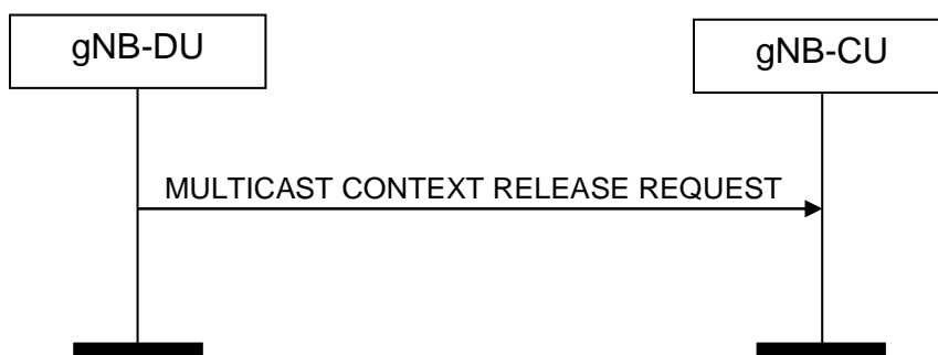
Figure 8.14.8.2-1: Multicast Context Release Request procedure. Successful operation
