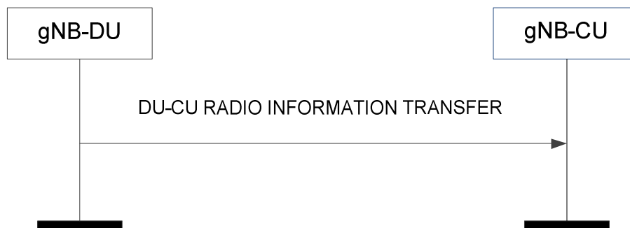
Figure 8.9.1.2-1: DU-CU Radio Information Transfer procedure.
