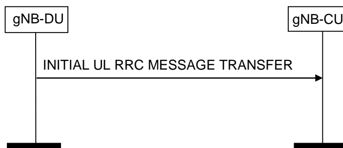
Figure 8.4.1.2-1: Initial UL RRC Message Transfer procedure.
