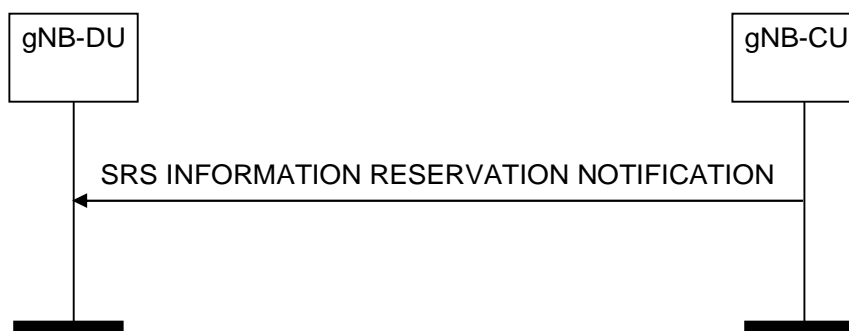
Figure 8.13.21.2-1: SRS Information Reservation Notification procedure, successful operation
