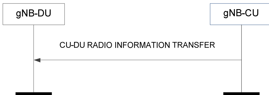
Figure 8.9.2.2-1: CU-DU Radio Information Transfer procedure.
