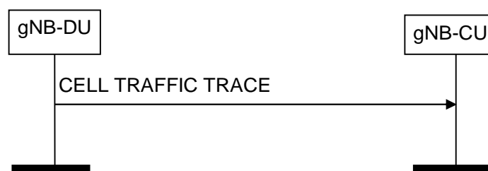
Figure 8.8.3.2-1: Cell Traffic Trace procedure. Successful operation.
