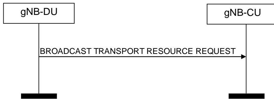
Figure 8.14.14.2-1: Broadcast Transport Resource Request procedure. Successful operation
