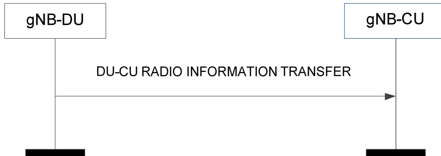
Figure 8.9.1.2-1: DU-CU Radio Information Transfer procedure.
