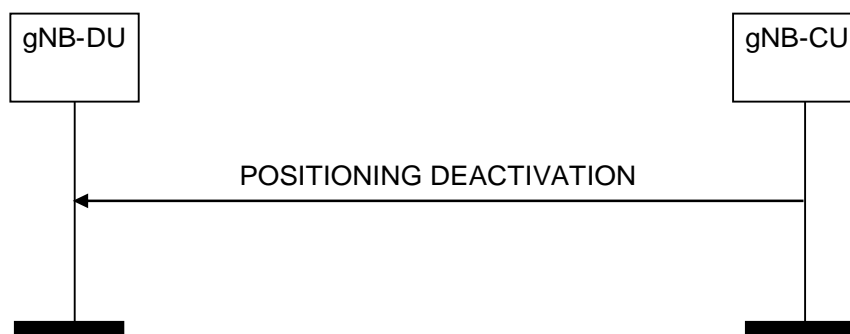
Figure 8.13.11.2-1: Positioning Deactivation procedure, successful operation
