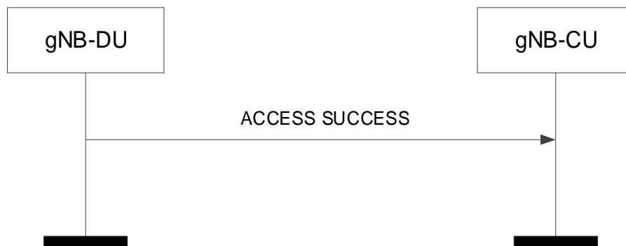
Figure 8.3.8.2-1: Access Success procedure. Successful operation.
