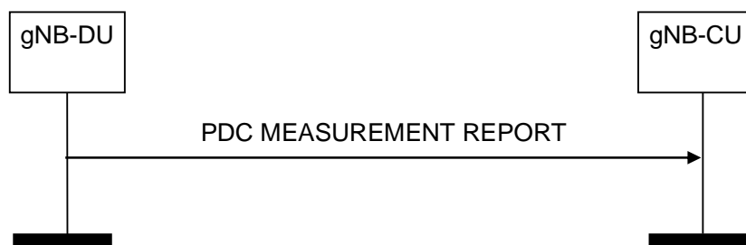
Figure 8.15.2.2-1: PDC Measurement Report procedure, successful operation
