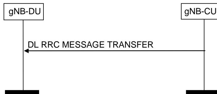
Figure 8.4.2.2-1: DL RRC Message Transfer procedure
