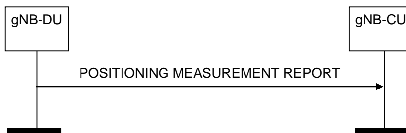
Figure 8.13.4.2-1: Positioning Measurement Report procedure: successful operation
