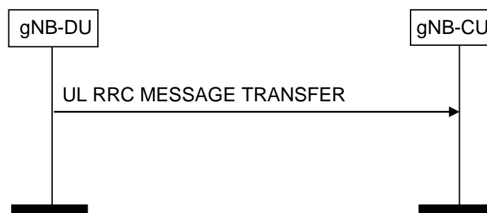
Figure 8.4.3.2-1: UL RRC Message Transfer procedure
