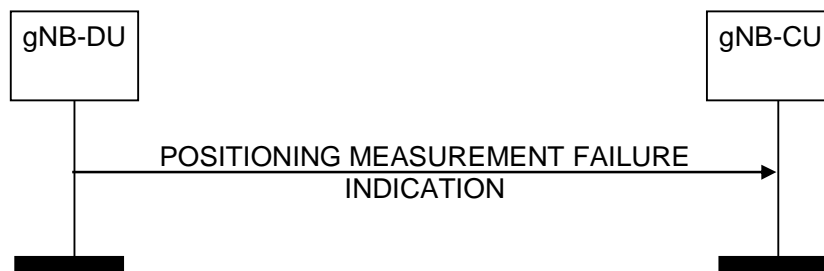
Figure 8.13.6.2-1: Positioning Measurement Failure Indication procedure: successful operation
