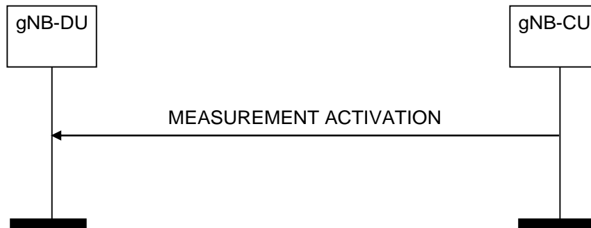
Figure 8.13.19.2-1: Measurement Activation procedure, successful operation
