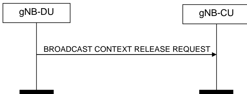
Figure 8.14.3.2-1: Broadcast Context Release Request procedure. Successful operation
