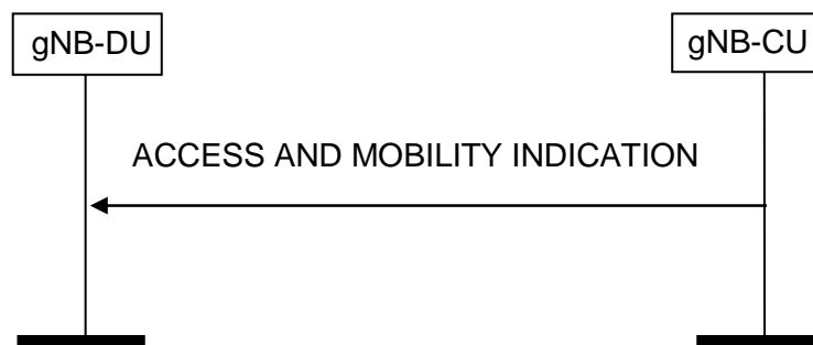
Figure 8.11.1.2-1: Access and Mobility Indication procedure. Successful operation
