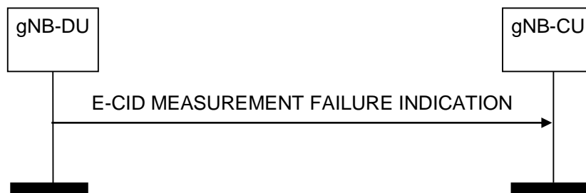
Figure 8.13.13.2-1: E-CID Measurement Failure Indication, successful operation
