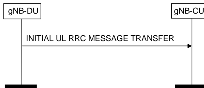
Figure 8.4.1.2-1: Initial UL RRC Message Transfer procedure.
