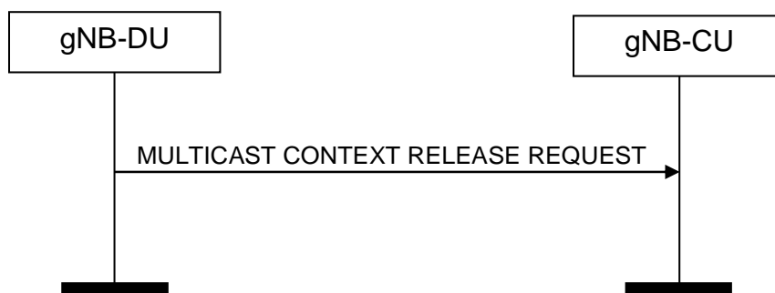
Figure 8.14.8.2-1: Multicast Context Release Request procedure. Successful operation
