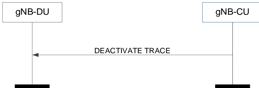
Figure 8.8.2.2-1: Deactivate trace procedure: Successful Operation
