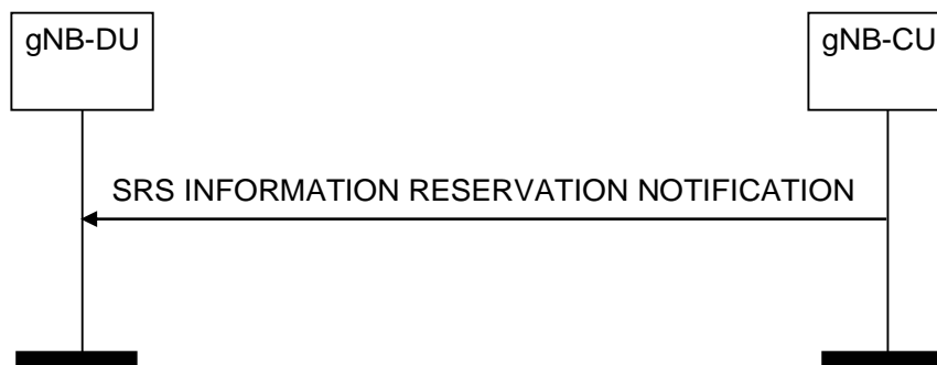
Figure 8.13.21.2-1: SRS Information Reservation Notification procedure, successful operation
