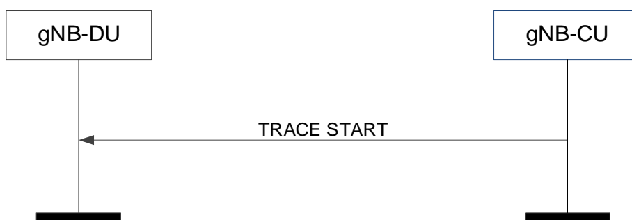
Figure 8.8.1.2-1: Trace start procedure: Successful Operation.
