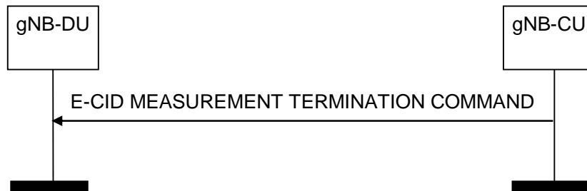
Figure 8.13.15.2-1: E-CID Measurement Termination procedure, successful operation
