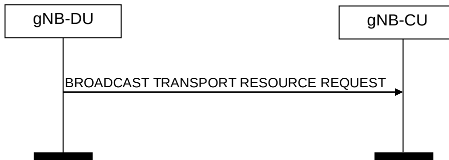
Figure 8.14.14.2-1: Broadcast Transport Resource Request procedure. Successful operation
