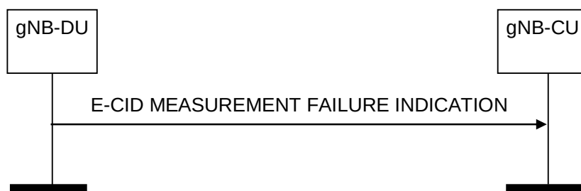
Figure 8.13.13.2-1: E-CID Measurement Failure Indication, successful operation
