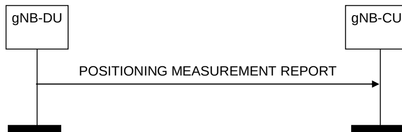
Figure 8.13.4.2-1: Positioning Measurement Report procedure: successful operation
