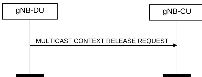
Figure 8.14.8.2-1: Multicast Context Release Request procedure. Successful operation
