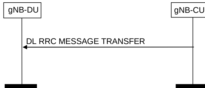
Figure 8.4.2.2-1: DL RRC Message Transfer procedure
