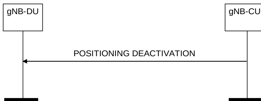
Figure 8.13.11.2-1: Positioning Deactivation procedure, successful operation
