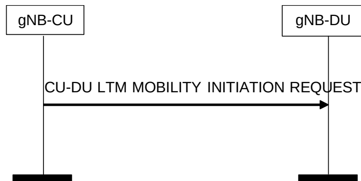
Figure 8.3.11.2-1: CU-DU Mobility Initiation procedure. Successful operation.
