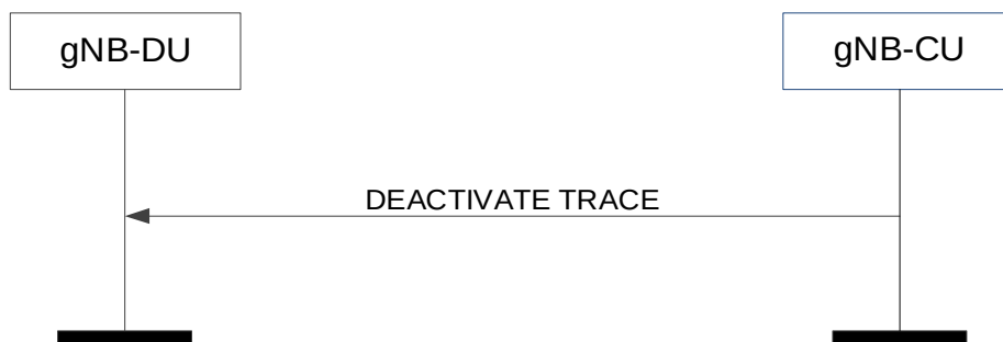
Figure 8.8.2.2-1: Deactivate trace procedure: Successful Operation
