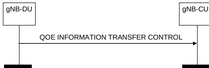
Figure 8.16.2.2-1: QoE Information Transfer Control procedure.
