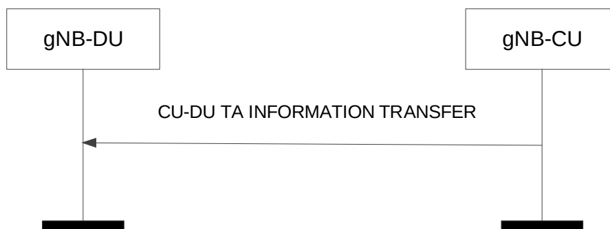
Figure 8.2.13.2-1: CU-DU TA Information Transfer procedure. Successful operation.
