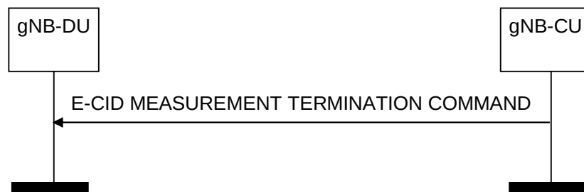
Figure 8.13.15.2-1: E-CID Measurement Termination procedure, successful operation
