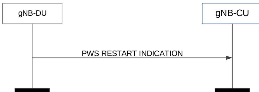
Figure 8.5.3.2-1: PWS restart indication
