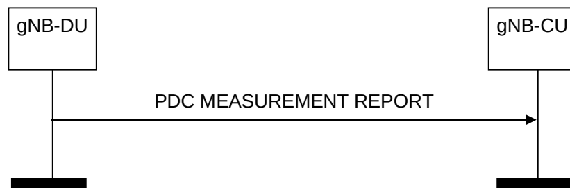
Figure 8.15.2.2-1: PDC Measurement Report procedure, successful operation
