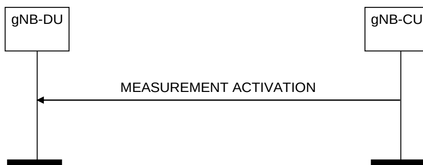
Figure 8.13.19.2-1: Measurement Activation procedure, successful operation
