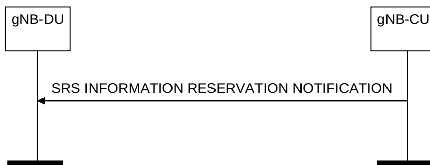
Figure 8.13.21.2-1: SRS Information Reservation Notification procedure, successful operation
