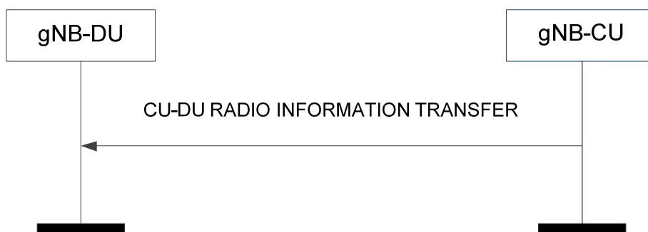
Figure 8.9.2.2-1: CU-DU Radio Information Transfer procedure.
