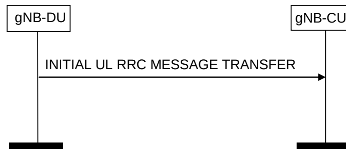
Figure 8.4.1.2-1: Initial UL RRC Message Transfer procedure.
