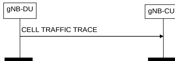
Figure 8.8.3.2-1: Cell Traffic Trace procedure. Successful operation.
