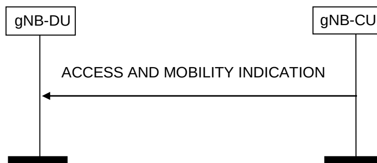
Figure 8.11.1.2-1: Access and Mobility Indication procedure. Successful operation
