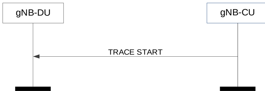
Figure 8.8.1.2-1: Trace start procedure: Successful Operation.
