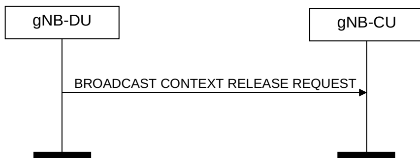
Figure 8.14.3.2-1: Broadcast Context Release Request procedure. Successful operation
