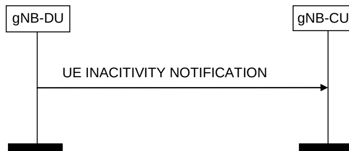
Figure 8.3.6.2-1: UE Inactivity Notification procedure.
