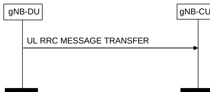
Figure 8.4.3.2-1: UL RRC Message Transfer procedure
