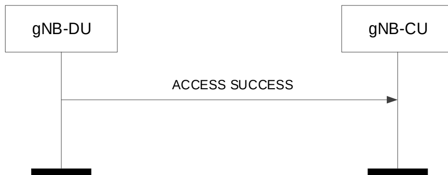
Figure 8.3.8.2-1: Access Success procedure. Successful operation.
