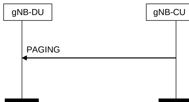
Figure 8.7.1.2-1: Paging procedure. Successful operation.
