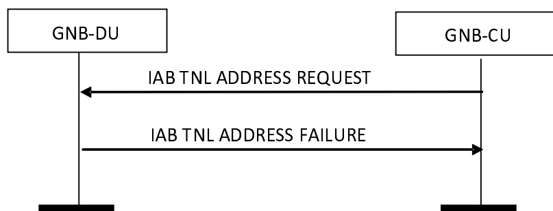
Figure 8.10.3.3-1: IAB TNL Address Allocation procedure: Unsuccessful Operation
