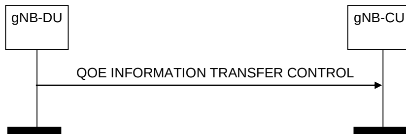
Figure 8.16.2.2-1: QoE Information Transfer Control procedure.
