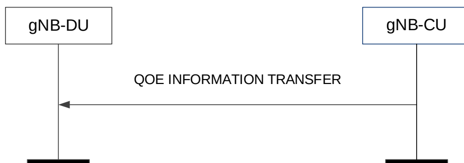
Figure 8.16.1.2-1: QoE Information Transfer procedure
