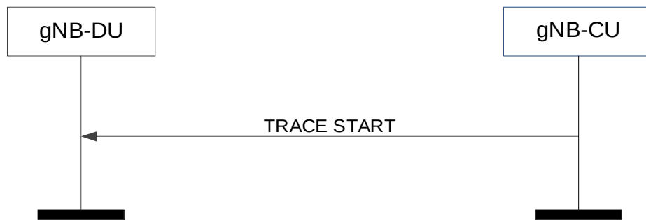
Figure 8.8.1.2-1: Trace start procedure: Successful Operation.
