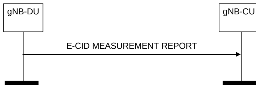
Figure 8.13.14.2-1: E-CID Measurement Report procedure, successful operation
