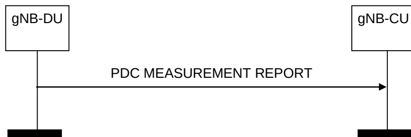
Figure 8.15.2.2-1: PDC Measurement Report procedure, successful operation
