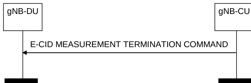
Figure 8.13.15.2-1: E-CID Measurement Termination procedure, successful operation
