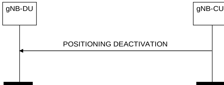
Figure 8.13.11.2-1: Positioning Deactivation procedure, successful operation
