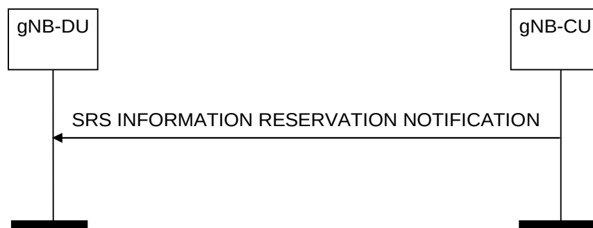
Figure 8.13.21.2-1: SRS Information Reservation Notification procedure, successful operation
