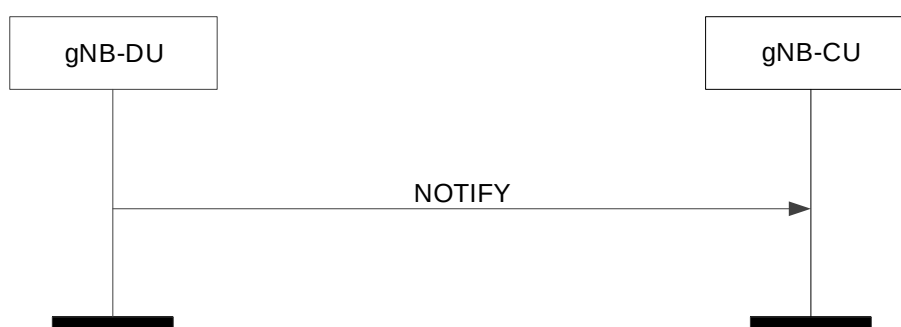
Figure 8.3.7.2-1: Notify procedure. Successful operation.
