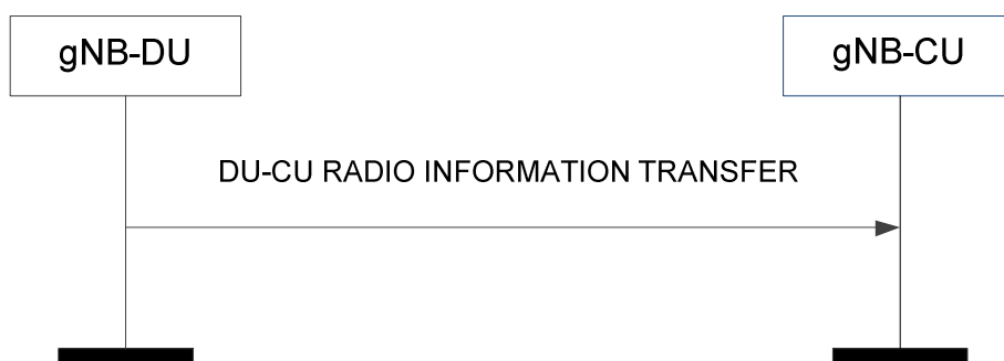
Figure 8.9.1.2-1: DU-CU Radio Information Transfer procedure.
