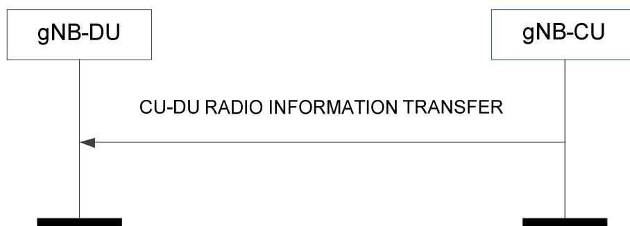
Figure 8.9.2.2-1: CU-DU Radio Information Transfer procedure.
