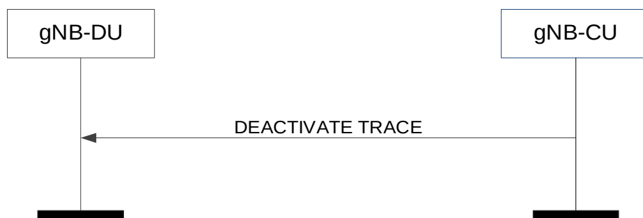
Figure 8.8.2.2-1: Deactivate trace procedure: Successful Operation
