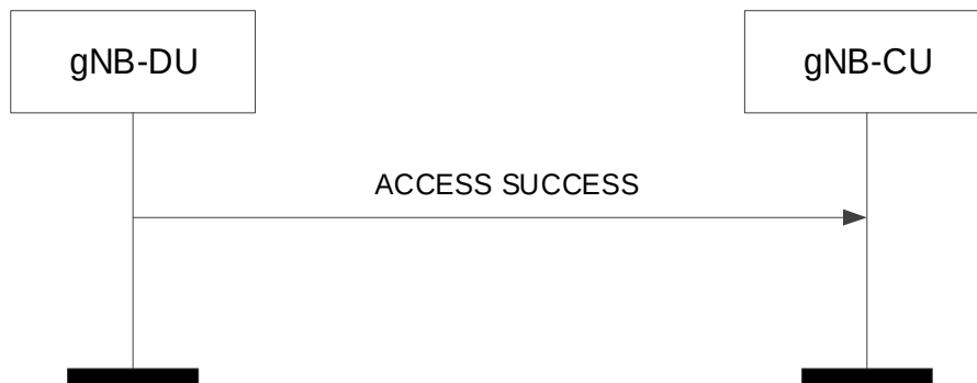
Figure 8.3.8.2-1: Access Success procedure. Successful operation.
