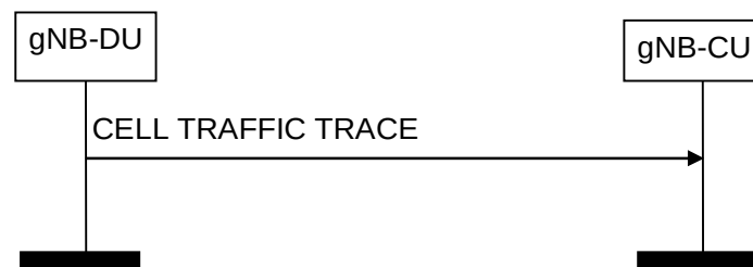
Figure 8.8.3.2-1: Cell Traffic Trace procedure. Successful operation.
