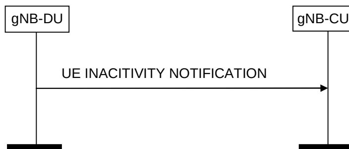
Figure 8.3.6.2-1: UE Inactivity Notification procedure.
