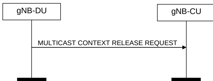
Figure 8.14.8.2-1: Multicast Context Release Request procedure. Successful operation
