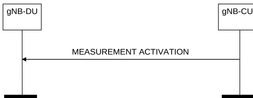
Figure 8.13.19.2-1: Measurement Activation procedure, successful operation
