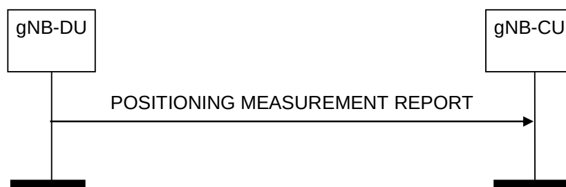
Figure 8.13.4.2-1: Positioning Measurement Report procedure: successful operation
