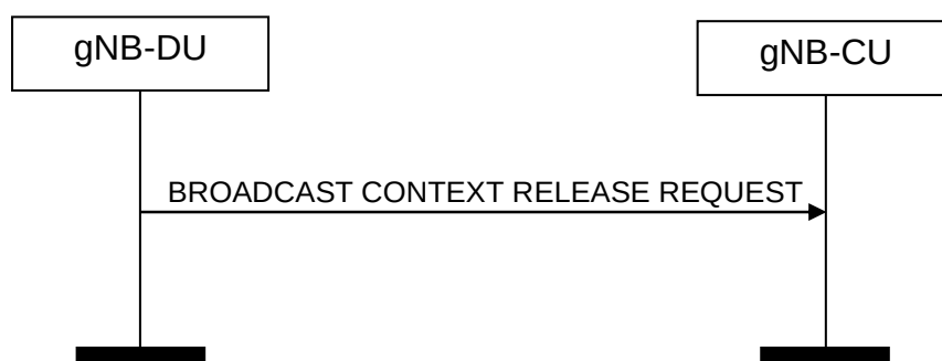
Figure 8.14.3.2-1: Broadcast Context Release Request procedure. Successful operation
