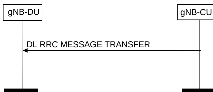
Figure 8.4.2.2-1: DL RRC Message Transfer procedure
