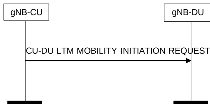
Figure 8.3.11.2-1: CU-DU Mobility Initiation procedure. Successful operation.
