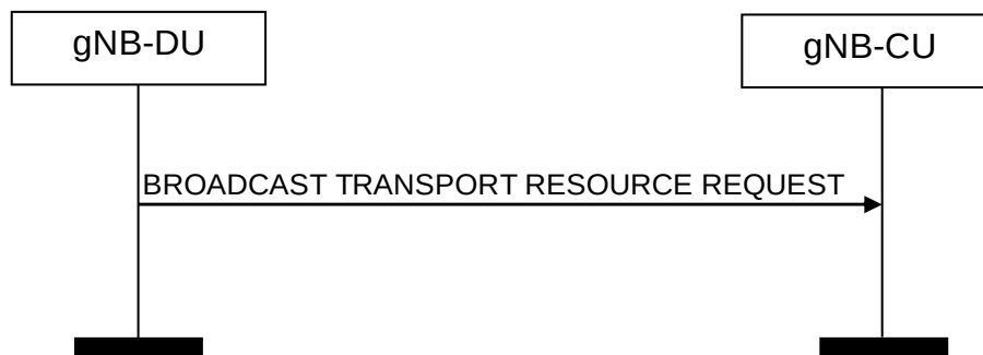
Figure 8.14.14.2-1: Broadcast Transport Resource Request procedure. Successful operation
