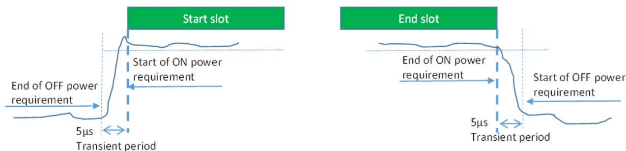
Figure 6.3.3.2.3-1: General ON/OFF time mask for NR UL transmission in FR2
